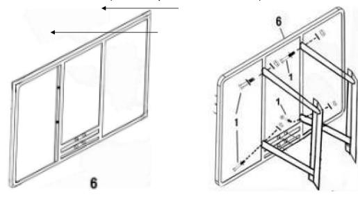
**Step 2.** Hold the backboard against your chosen wall and position it as required (you will need two people to do this) then using a pencil or marker, draw through the holes on the bracket to mark where holes need to be drilled.
