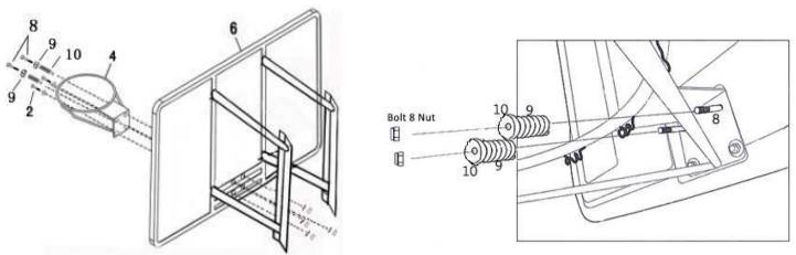
**Step 4:** Fix the backboard brackets to the wall using the raw bolts (item 3). Drill holes in your wall to the required depth, and then insert the raw bolts with the nuts facing outwards. Remove the nut, place the backboard onto the bolts and fix on with the nuts. The raw bolt will expand as you tighten to secure the backboard, please see diagram below for further advice.
