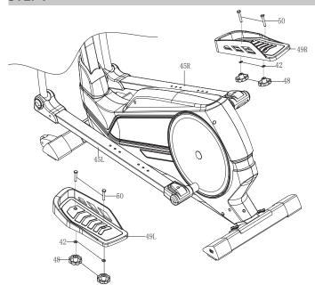
• Attach the pedals (49L & 49R) to the pedal arms (45) with bolts (50), washers (42) and nuts (48).
