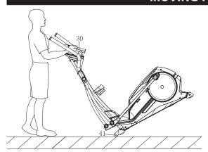
To move the machine, press on the middle handle-bar (30) until the transportation wheels on the front stabilizer (41) touch the ground. With the wheels on the ground, you can transport the bike to the desired location with ease.
