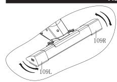
When this machine is placed on an uneven surface, please adjust both foot pads on end cap (109L/R) according to the drawing on the left until it is perfectly stabilized.
