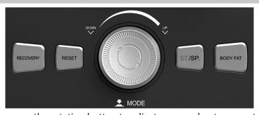
UP/DOWN: You can use the rotating button to adjust your workout parameters, or while exercis-
