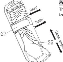
The strap (27) on the pedals (25) is adjustable and can be personalized to fit the user's foot size.
