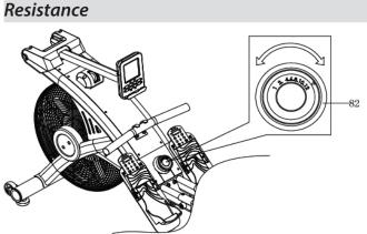
Rotate the tension knob (82) **clockwise** (the same as the clock's hands) to **increase** the resistance, or **counterclockwise** (the opposite of the clock's hands) to **decrease** the resistance. The range is between «1» (minimum) to «12» (maximum).
