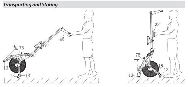
To move the rower, lift if by the rear support (46) until the wheels (13) on the front support (18) touch the ground. You can then easily transport it wherever you want (left drawing).
