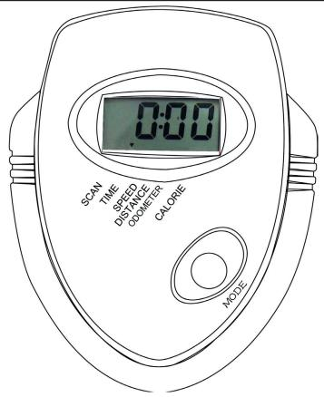
The console will automatically turn on when you start pedaling. It will also turn off by itself, after 4 minutes of inactivity.
