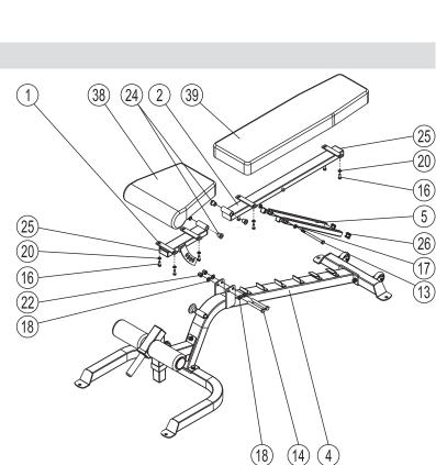
secure using four M8 x 25 Bolts (16) and M8 Washers (20).
