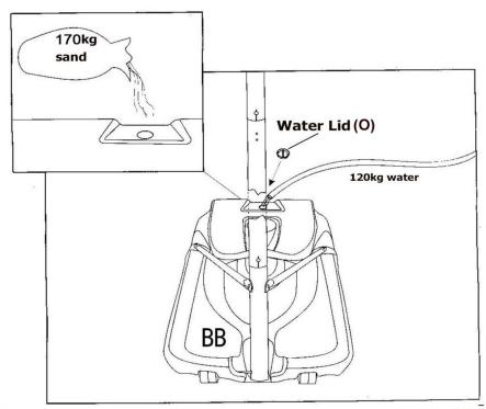
For safety reasons sand instead of water is recommended to fill up the tank. If a small leak develops, water might run away unnoticed, allowing the stand to fall over causing personal injury and/or death or property damage. Place the base on a smooth surface only, away from sharp objects that might be able to puncture it.
